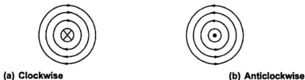
Fig. 3.16 Representation of direction of flux
